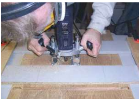
▲ Pic.8 Make a jig for cutting the housings in the sides for the drawer runners/kickers
